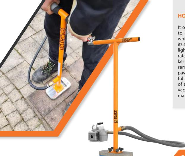
It only takes one person to operate the device, which is characterised by its small size. The device is light and handy. It is operated by pressing the sucker against the stone, then removing the damaged paving stone with a careful movement. It consists of a handle, sucker and vacuum pump. It is 230 V mains powered.
