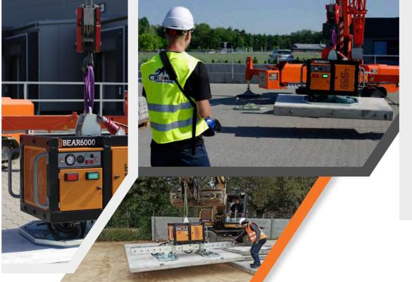
The Bear6000 is used to lift, move, rotate and plumb all kinds of concrete slabs and precast concrete products weighing up to 6000 kg. It consists of an oil-driven vacuum pump driven by a combustion or electric motor from a 400V network. The electric version enables operation indoors and allows for suspension from the crane.
